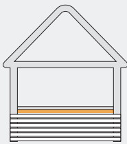
Sub-floor with timber battens
